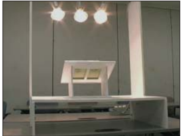
A bank of infrared lamps is arranged to shine on test materials mounted at an angle approximating a roof exposure.
